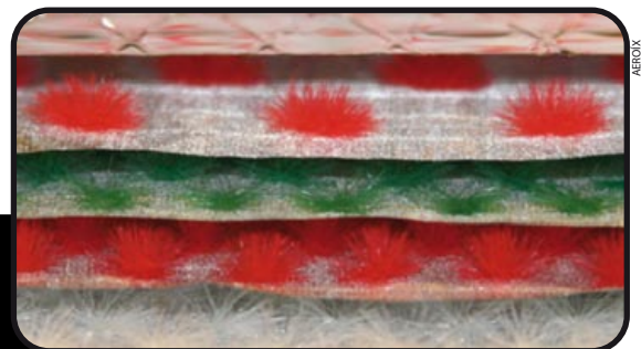
Close-up of different variants of the aerofabrix® flock insulation
