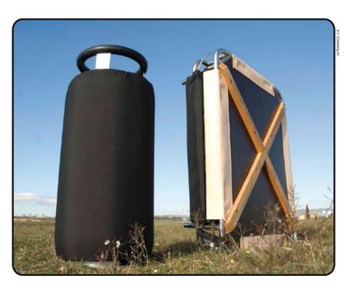
The fold down **Tekno** basket weighs in at less than 35 kg and is capable of flying two people with a range of cylinder configurations. The side walls are made of a combination of durable Cordura covers filled with light weight composite materials giving a firm feeling of security whilst also being able to fold down into a very compact package.
