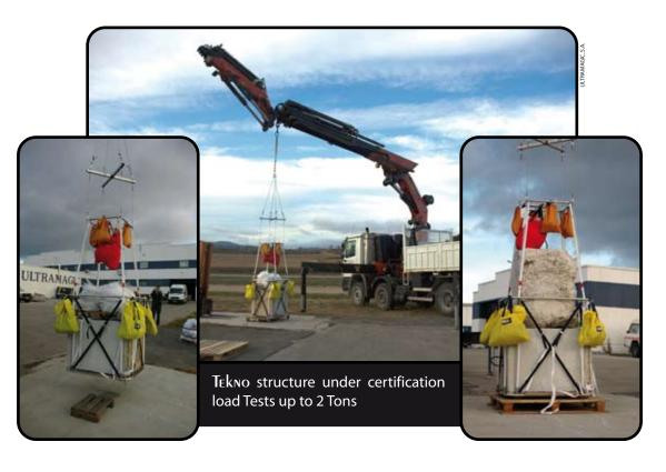
The **Tekno** basket has been extensively tested to meet the harshest of operational conditions!
