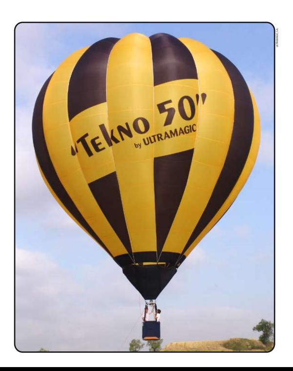
The super light weight 50,000 ft<sup>3</sup> **Tekno 50** envelope weighs less than 50 kg including bag. This 16 gore 8 wire easy to inflate envelope packs down into a bag no larger than that normally used for a 31! Made complete with Ultralite fabric the envelope uses the latest light weight Kevlar load tapes as well as a number of other innovative weight saving materials.
